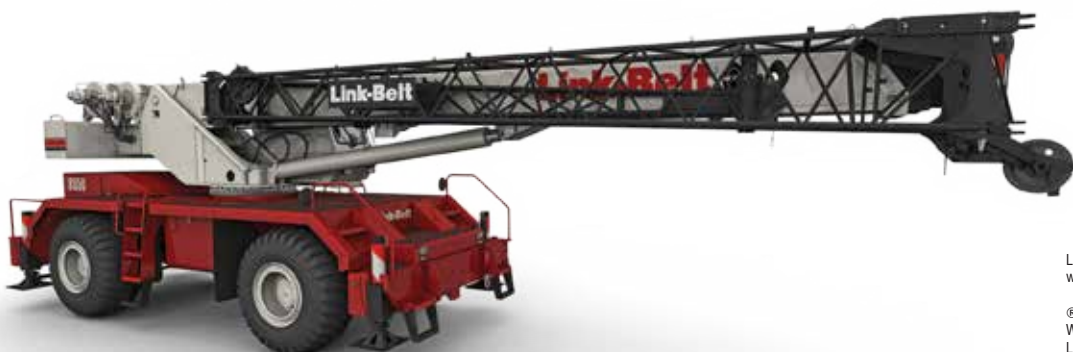
A-max extends only the inner-mid section of the boom for substantially increased capacities for in-close, maximum capacity lifts.
