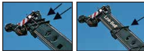
A-max extends only the inner-mid section of the boom for substantially increased capacities for in-close, maximum capacity lifts.
