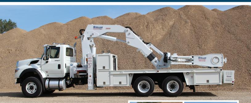
The Stellar 28000 OTR series tire service crane fits the need of OTR tire service technicians who need something that can handle it all. A 320-degree turntable rotation system driven by a worm gear / pinion system ensures rock solid performance. This crane features a lifting capacity of 28,000 lbs. at 10' and 17,200 lbs. at 16'3" of total reach, without the tire manipulator.
