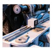
Mounting rail allows attachment of camera, lights, and other accessories using Unistrut hardware.
