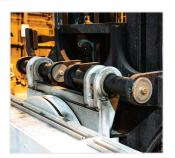
Side shift allows for 8" of left movement and 8" of right movement to align tire to hub. (Optional)
