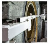
Hydraulic fall back protection and ring catcher arms holds tire in place and allows for easy removal of lock ring components.
