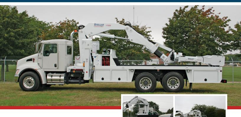
Designed from the ground up to provide maximum lifting performance and solid stability, the Stellar® 17000 is the largest OTR crane in the industry allowed on a single axle truck. It also offers over 18' of stabilizer spread to keep your truck stable.
