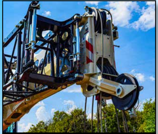
Quick reeve boom head eliminates the need to remove the becket when it becomes necessary to change the reeving.
