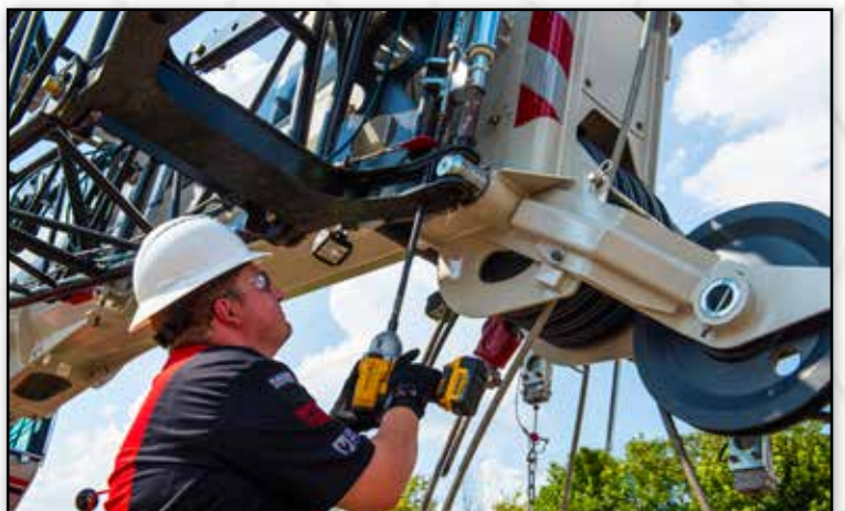
Link-Belt's patented fly erection system is designed for safe and simple assembly. Boom head speed screws aid in quick, reliable fly erection and stowage
